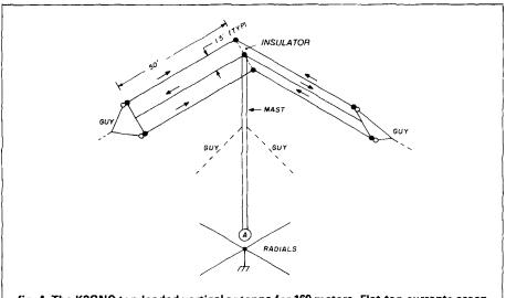
fig. 4. The K2GNC top-loaded vertical antenna for 160 meters. Flat-top currents essentially cancel and majority of radiation comes from 88-foot vertical element. Antenna is base-fed at point A via coaxial line and simple L-network. Spacing between wires is about a foot.
